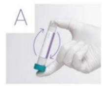
Mix the sample by gently inverting the tube 5 times.
