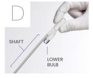
Ensure the **shaft** is filled with liquid sample. Note: Do not squeeze lower bulb or invert the pipette.
