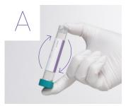
Mix the sample by **gently** inverting the tube 5 times. Note: Failure to invert may lead to inaccurate results.
