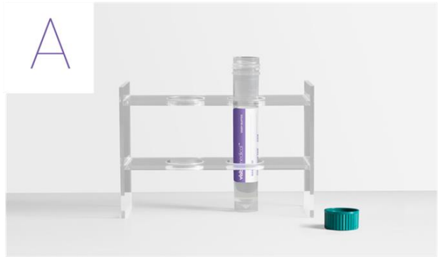
Open the Visby Respiratory Health Buffer Tube and place it in a tube holder.
