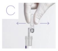
Release the upper bulb slowly to fill the shaft. Keep pipette tip submerged until shaft is full. Extra fluid should enter the lower bulb.
