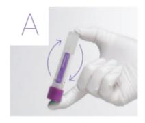
Mix the sample (or control) by **gently inverting** the tube **5 times**.
