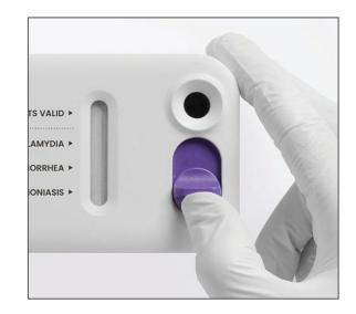
123Plug in DevicePipette SamplePush Port Closed
