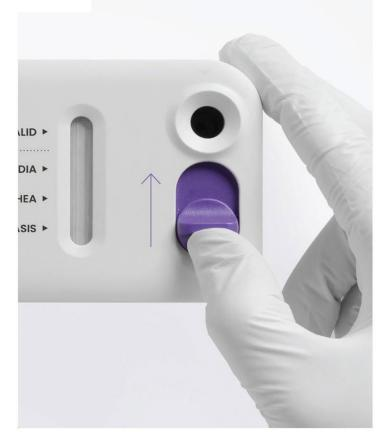
Immediately after sample addition, slide the **switch upwards** in a firm, swift motion to fully close the sample port and ensure the test is started.
