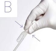
Squeeze the **upper bulb** of the provided pipette and submerge the tip to the **bottom** of the sample tube.
