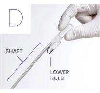
Check that there are **no air bubbles** in the shaft. **Note:** Do not squeeze lower bulb or invert the pipette.
