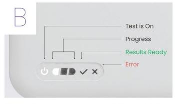
Check that the first progress **indicator light is blinking**. Lights will initially blink and then become stable as the test progresses.
