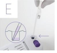
Place the tip at the **bottom** of the sample port and then squeeze the **upper bulb** of the pipette to release **all** of the sample.
