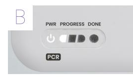
Check that the first progress indicator light **is blinking**. Lights will initially blink and then become stable as the test progresses. Note: If something different happens to the lights, please refer to the Troubleshooting Section.
