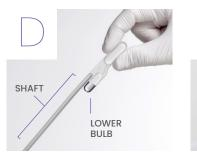
Ensure the **shaft** is filled with liquid sample. Note: Do not squeeze lower bulb or invert the pipette.
